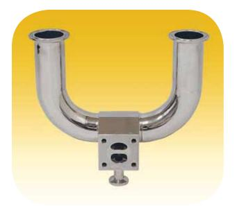
The Zero DL<sup>®</sup> Point-of-Use Valve utilizes the T-pattern design to promote efficient installation when used on clean water loops. The main valve body is machined from a solid block of 316L stainless steel. It's design improves drainability and eliminates deadlegs within a processing system. Available in valve sizes 1/2" to 4" with tubing run sizes through 6" in clamp , buttweld ends, and other specialty connections.
