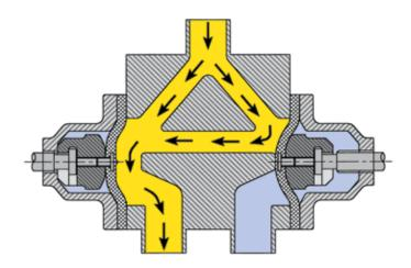
The flow pattern on the closed side of the valve will allow for a continuous flow to the open side providing zero deadleg.
